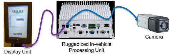
Figure 2. The key hardware components of the tooth guard system include 1) a camera mounted on the boom of a shovel; 2) a computational processing unit ruggedized in the vehicle; and 3) a display unit in front of the operator.
