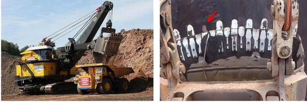
(a) A rope mining shovel (b) A bucket with a missing tooth
